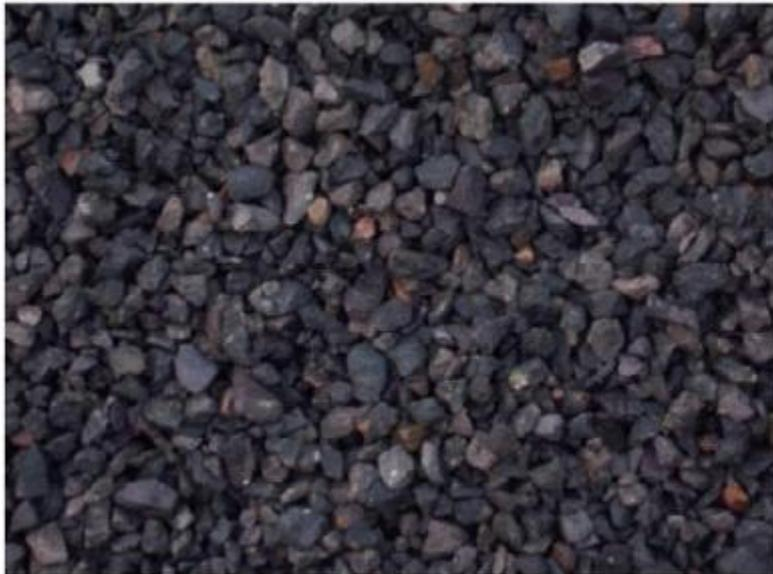
**(b) Recycled coarse aggregate for concrete**
